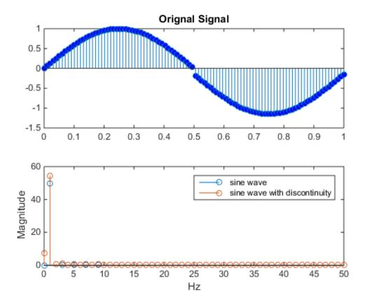
There is minimal difference in the magnitudes of the Fourier coefficients. Because the discrete Fourier basis vectors have support over the entire time interval, the discrete Fourier transform does not detect the discontinuity as efficiently as the wavelet transform.
