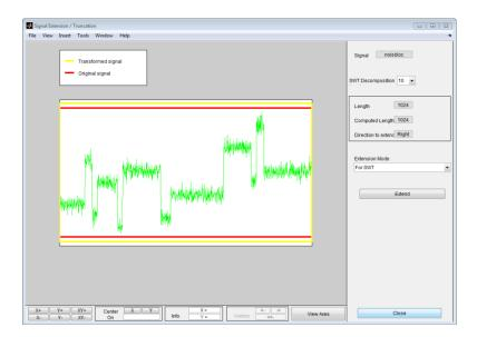
Since the signal is of length  $1024 = 2^10$ , no extension is needed so the **Extend** button is ineffective.
