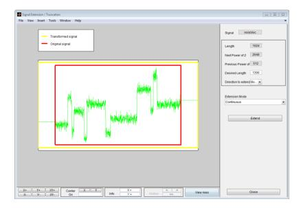
The signal is extended in both directions by replicating the first value to the left and the last value to the right, respectively.
